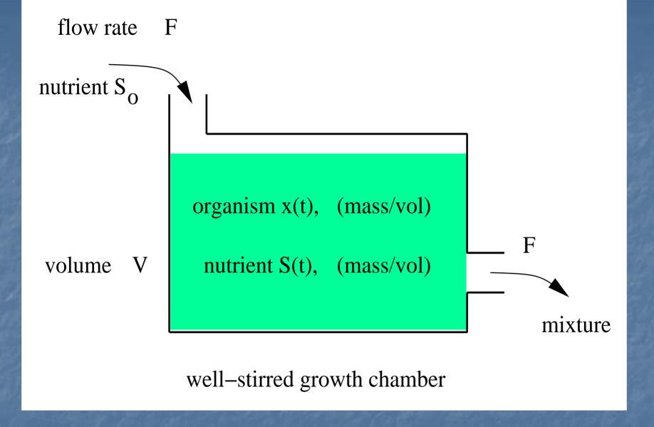
dx/dt = rate produced - rate out
