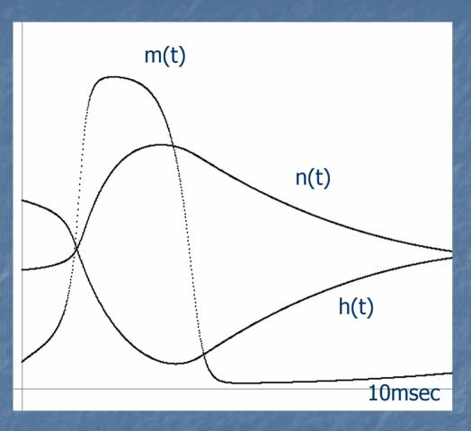
$\rho_m(v)$  dm/dt =  $m_\infty(v)$  - m.  $\rho_m(v)$  is much smaller than  $\rho_n(v)$  and  $\rho_h(v)$ . An increase in v results in an increase in  $m_\infty(v)$  and a large dm/dt. Hence Na activates more rapidly than K in response to a change in v.
